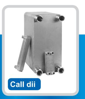
The compact size, low refrigerant charge, and superior heat transfer characteristics of Doucette's Brazed Plate Heat Exchangers make them ideal for evaporator, condenser and sub-cooler applications. Available for virtually any duty, the Brazed Plate Heat Exchangers are available with copper or nickel brazing materials. Standard units have 316 Stainless Steel plates with copper brazing and sweat connections. U.L. listed for 650 psig DWP.
